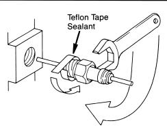
Use of threaded connections in a vacuum system should be minimized. The small spaces between the threads will cause virtual leaks. If threaded connection must be used, one of the connections should be slotted to permit rapid pumping of the threads and blind hole, if any.
