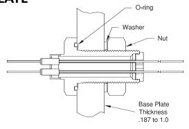
Install feedthrough with o-ring on vacuum or pressure side of the wall. Place washer and nut on air side of system. Tighten nut to compress o-ring.
